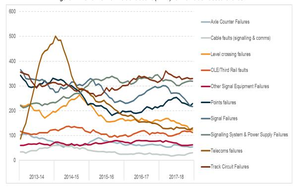
Figure 7 – Overview of incident count (MAA) for non-track asset failures
