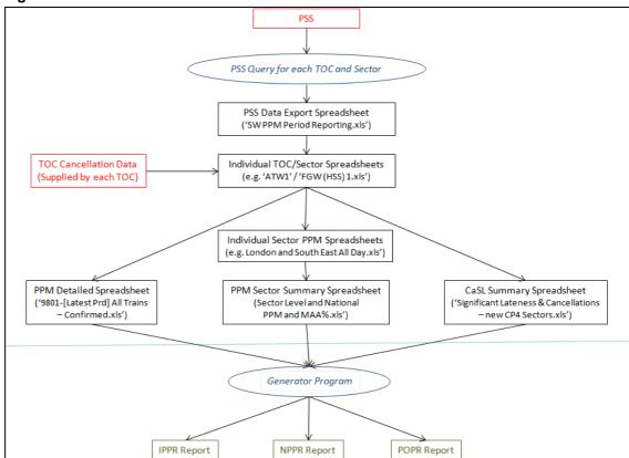
Figure 5.1: Data Process for PPM and CaSL
