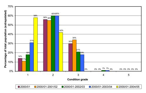
Figure 5.9.3 Average condition grades for DC sub-stations (M14)
