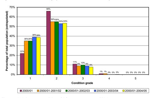
Figure 5.10.3 Average condition of AC contact systems (M14)
