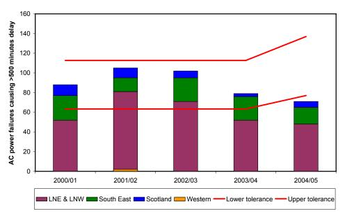
Figure 5.7.1 Number of AC power failures causing >500 minutes delay (M11)
