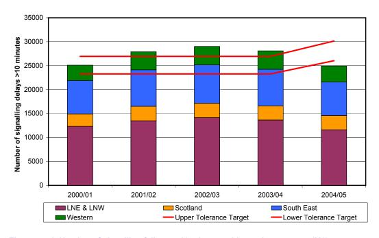
Figure 5.5.1 Number of signalling failures >10 minutes with regulatory target (M9)
