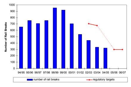
Figure 5.1.1 Number of broken rails (M1)
