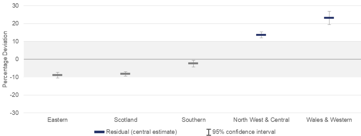
Figure 2: Deviation between outturn and expected (modelled) unit costs for conventional track renewals by Network Rail region, 2022-23
