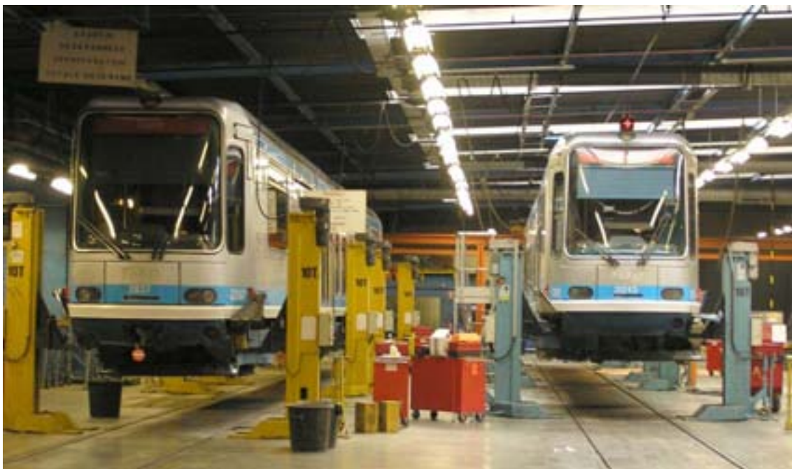
E Hollis (2020086) (b) Tram No. 2037 and 2013 lifted for work on bogies
