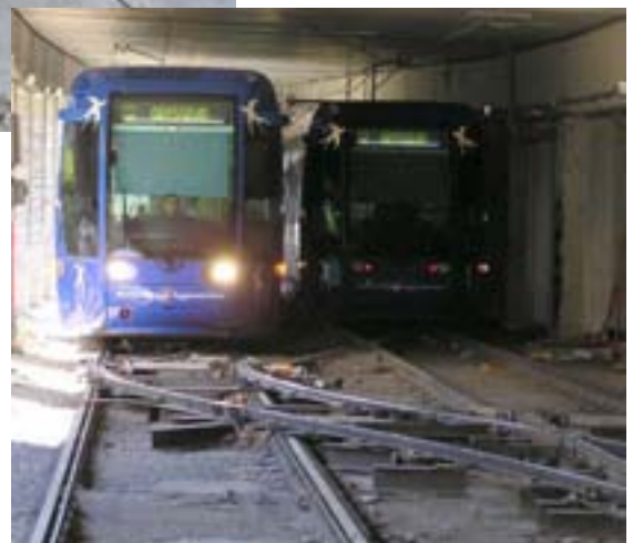
Figure 11.21 Temporary crossovers at Corum, TaM Montpellier (03.03.05)
