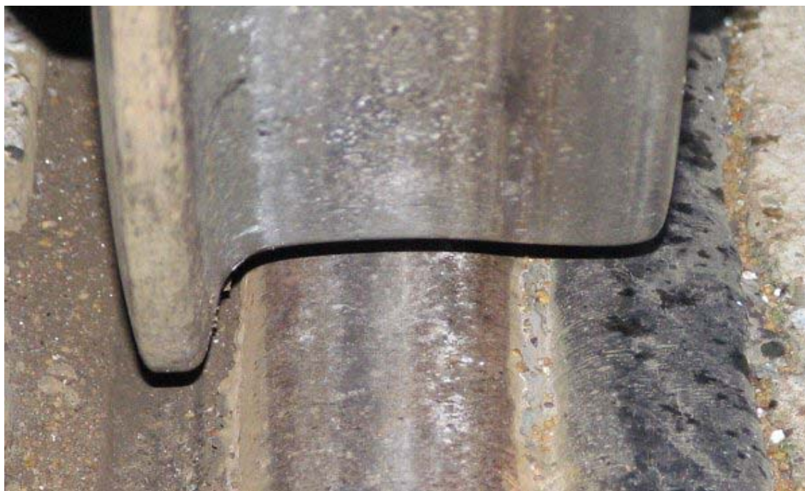
Figure 13.2 Example of an 'in service' wheel profile
