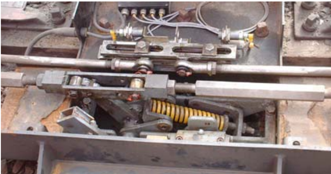
Figure 13.4 Example of a switch rail that has not been fully closed by the switch mechanism
