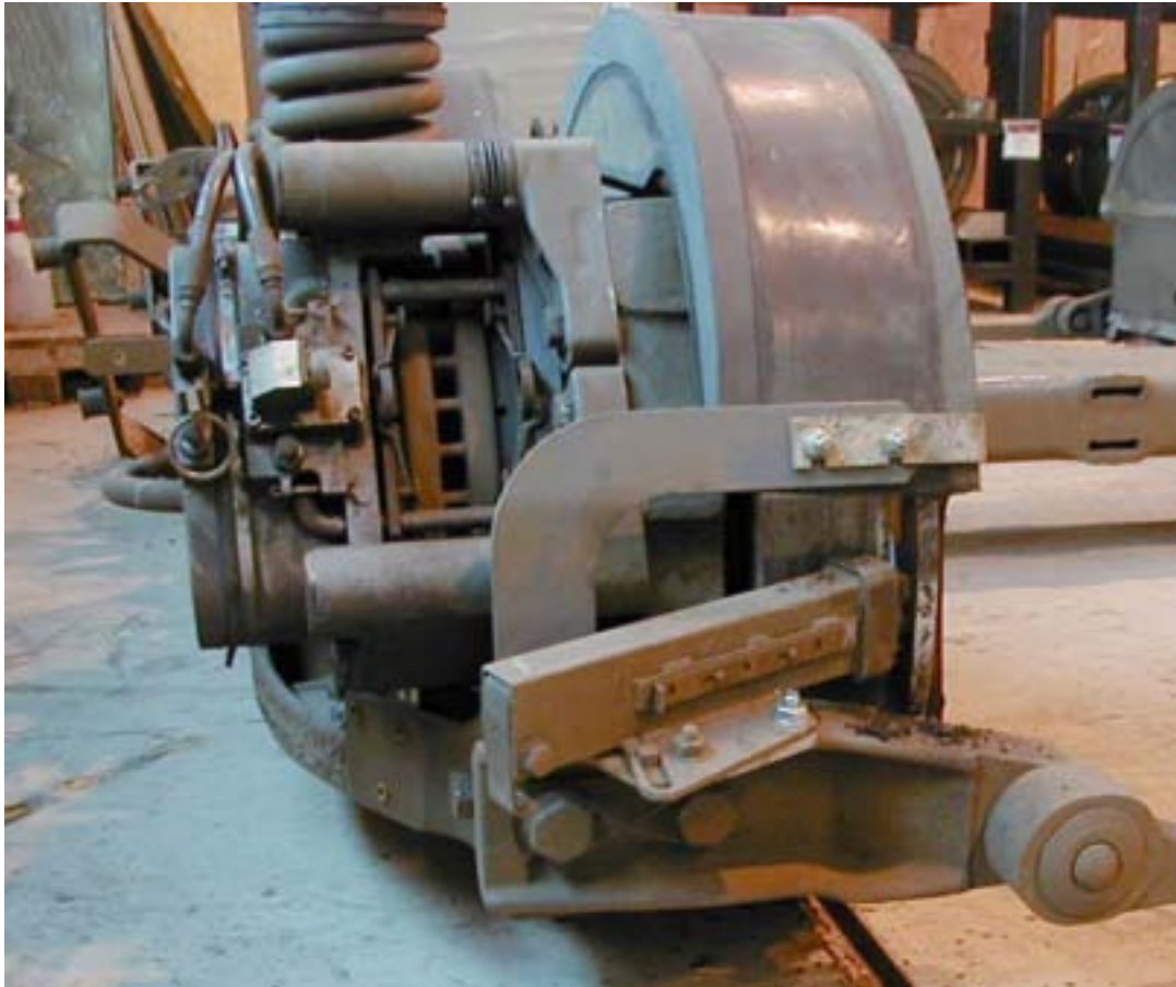
Figure 3.25 Trailer truck wheel/stub axle detail showing solid stick lubricator bearing on wheel flange root, Croydon Tramlink (12.02.04)
