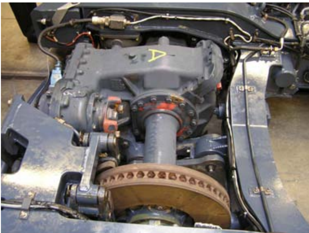
(b) Gearbox and brake detail
