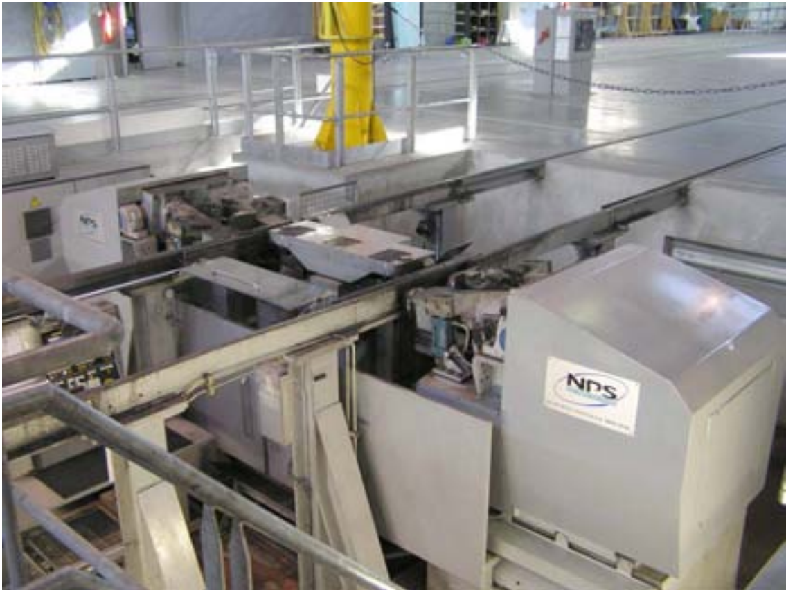
Figure 11.28 The TaM Montpellier wheel lathe at the Depot (03.03.05)
