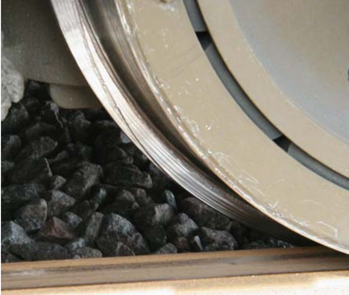
Figure 13.9 Wheel marks following a derailment
