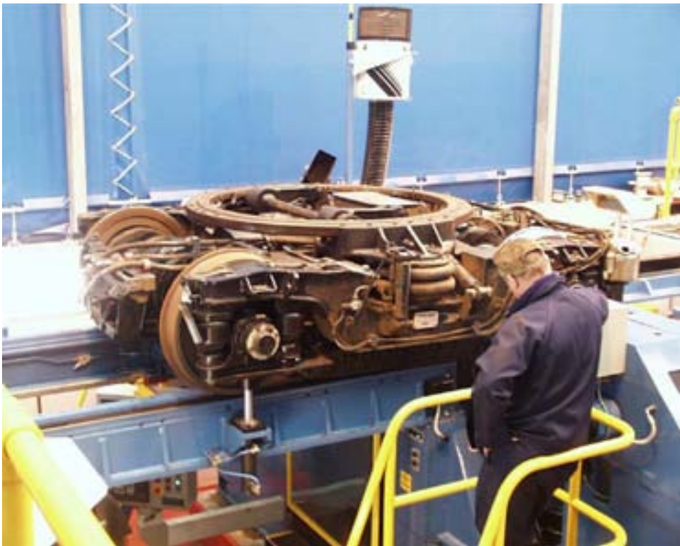
Figure 6.13 Midland Metro Firema M046 motor bogie on the wheel lathe
