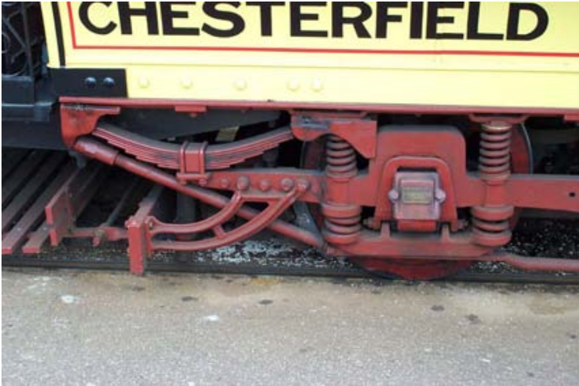
Figure 7.10 A P22 truck showing the primary coil and secondary leaf spring suspension, at The National Tramway Museum
