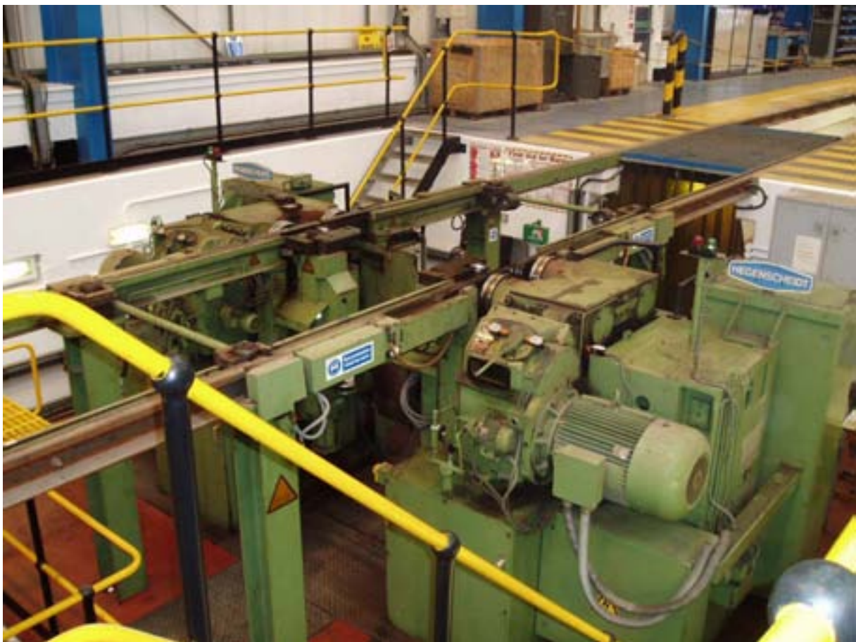
Figure 9.17 The SYS wheel lathe at the Depot (06.10.04)
