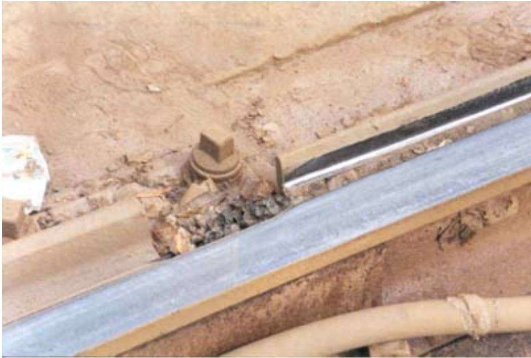
(a) Keeper flange wear
