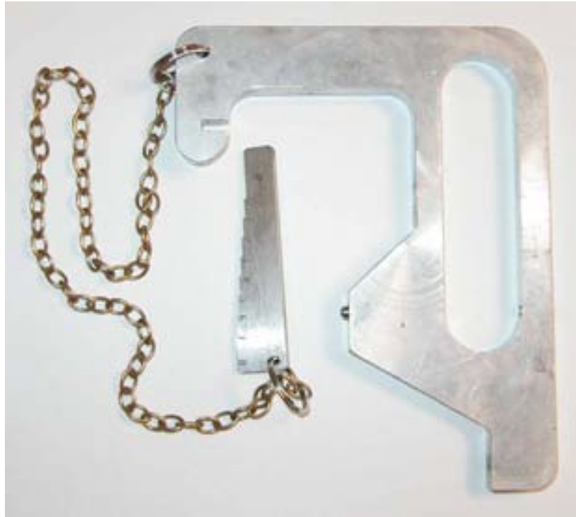
Figure 3.7 S 49 flat bottom rail wear gauge, Croydon Tramlink
