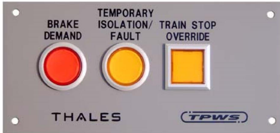
Figure 6 - Typical TPWS panel
