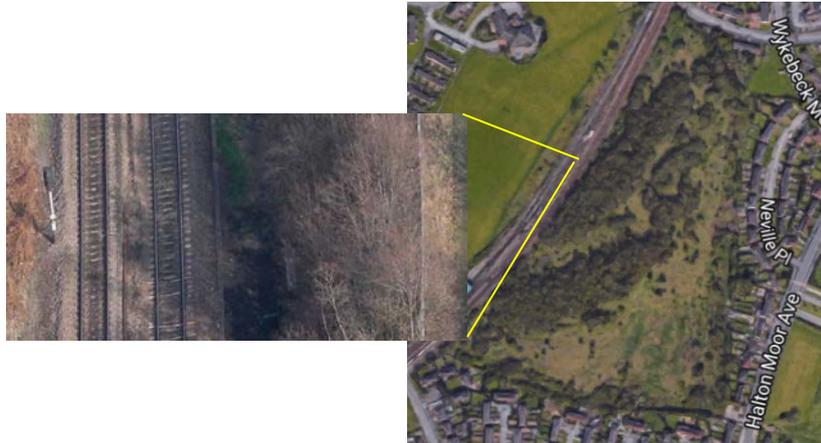
Figure 1 Aerial photograph showing existing twin track alignment centred on former 4 track alignment adjacent to former Waterloo Carriage Sidings.
