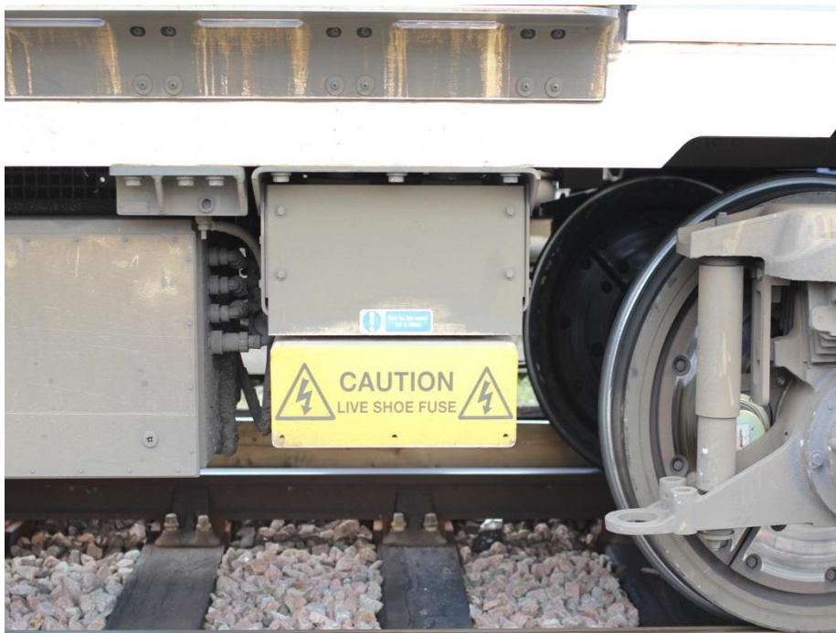
Simple cover fitted over shoe fuse
