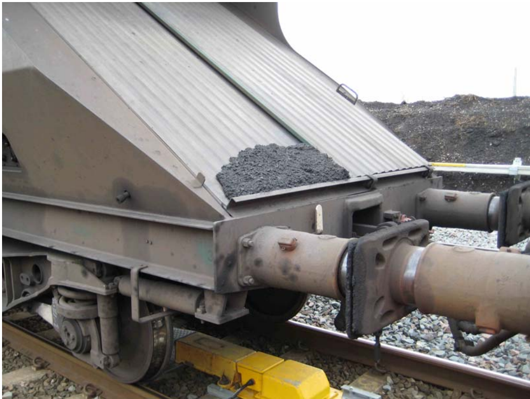
Above: Coal Spillage on Wagon end railing
