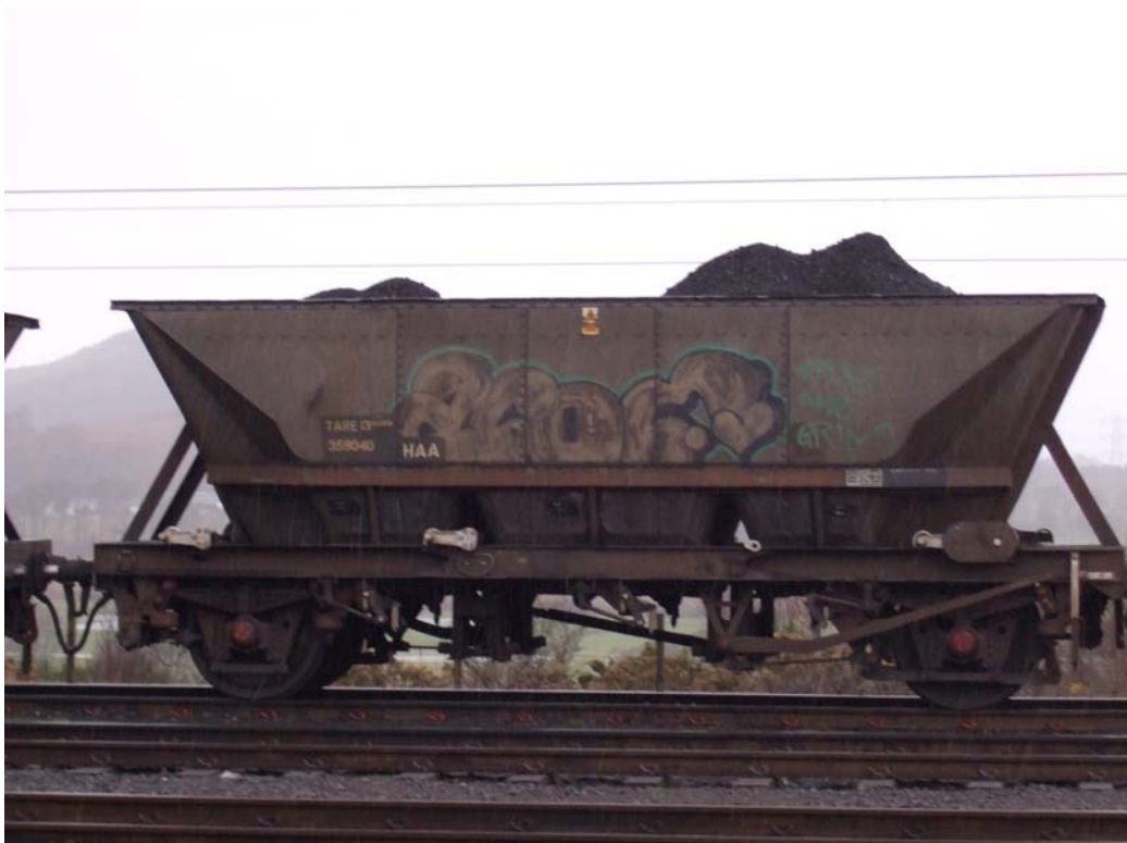
Above: Coal Spillage on Wagon end railing
