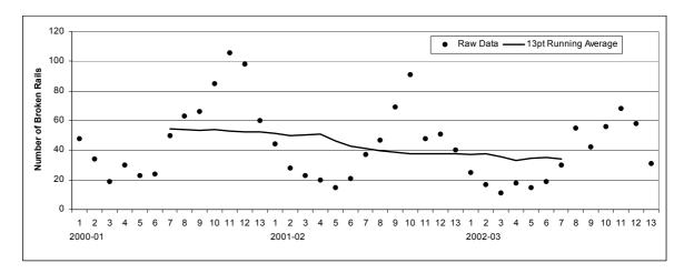
Figure 1. Trend in the Number of Broken Rails Identified.
