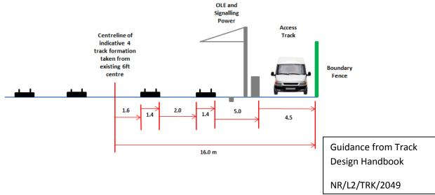
Figure 3 Outline dimensions used to calculate distance to boundary.
