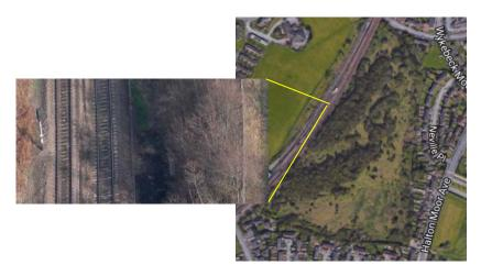
Figure 1 Arial photograph showing existing twin track alignment centred on former 4 track alignment adjacent to former Waterloo Carriage Sidings.
