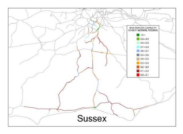
Diagram 20 Capacity of the Electrification Systems in MVA per STK (Network Rail)
