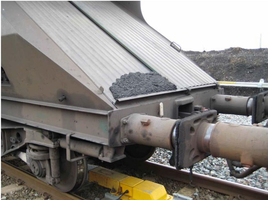
Above: Coal Spillage on Wagon end railing
