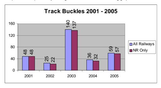
There is a strong correlation between high ambient temperature and the number of track buckles recorded. However, HMRI acknowledges the improved procedures Network rail has in place for monitoring the effects of high ambient temperatures on its infrastructure. Figures for 2005, while higher than those for 2004, are broadly consistent with previous years. The 2005 figures are significantly lower than the figures of 135 and 137 experienced during the long hot summers of 1995 and 2003.
