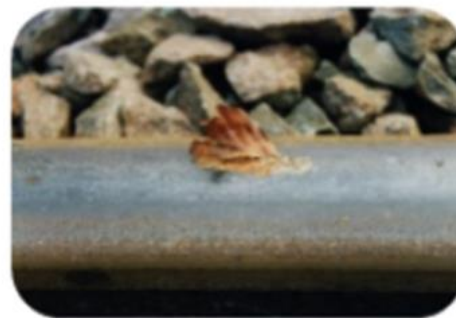
Leaves on the line make tracks slippery and affect connectivity
